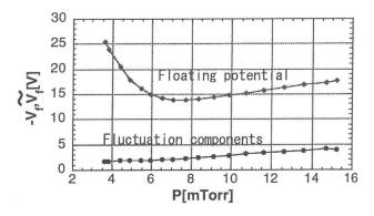
Fig.2. The averaged floating potential and its fluctuating components as a function of the neutral pressure.
