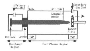
Fig.1. Schematic of experimental apparatus NAGDIS-II.
