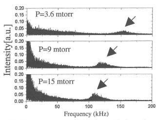
Fig.3 Frequency spectra of the electrostatic fluctuation as a parameter of the neutral pressure P
