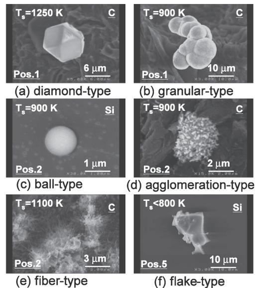
Fig. 2 SEM pictures of carbon dust on the graphite targets and silicon crystal targets.
