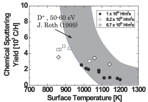
Fig. 1 Temperature dependence of chemical sputtering yield estimated by the weight loss of graphite targets.
