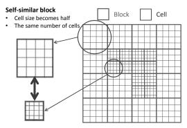
Fig. 1. Example of block configuration in two-dimensional domain. In this case, a block has 4×4 cells.
