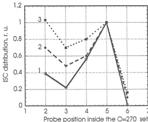
Fig.1. Ion saturation current distributions inside  $\Theta=180^\circ$  (a) and  $270^\circ$  (b) probe arrays.
