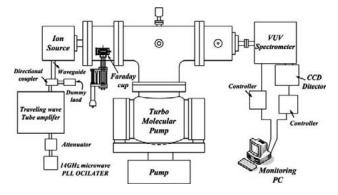
Fig. 1. The experimental setup used to measure the VUV spectrum emission from a 14 GHz ECR H<sup>-</sup> ion source.
