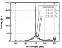
Fig. 2. The observed photon emission spectrum from a 14 GHz ECR H<sup>-</sup> ion source.
