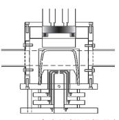
Fig. 3. The structure of a 2.45 GHz ECR H<sup>-</sup> ion source to compare the performance with a 14 GHz source. The diameter of the ceramic discharge chamber is 5 cm.
