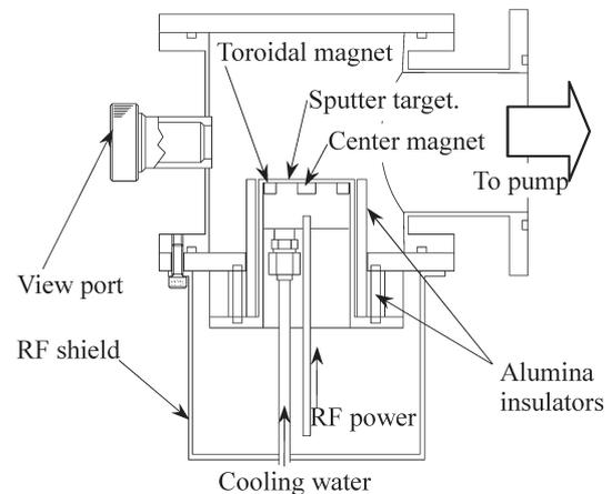
Fig. 1. A test mock-up assembled to investigate RF discharge at low pressure.
