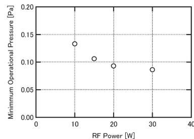
Fig. 2. Minimum Ar pressure required to sustain RF magnetron discharge.
