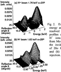
Fig. 2. Examples of energy and angular resolved intensity profiles of H<sup>+</sup> and ions reflected from Mo surface at the incident angle of 20o for (a)  $H^+$ and (b) H<sup>-</sup> beam
