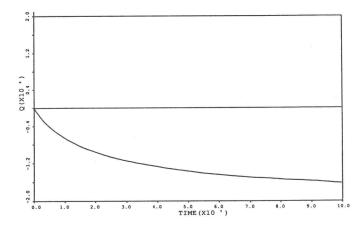
Fig.1. The temporal charging process of the grains when the secondary electron emission effect is neglected.
