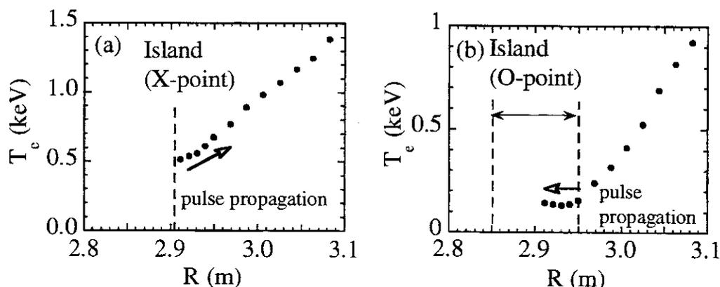
Fig.4 Radial profiles of electron temperature at the (a) X-point and (b) O-point of the magnetic island measured with ECE just before the TESPEL is injected.
